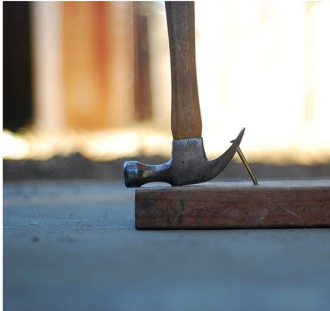
A hammer can be used to pull a nail out of a board. You can see how it's done in this picture. When you push down on the handle of the hammer, the claw end of the hammer pulls up on the nail. A hammer is an example of a machine called a lever.
