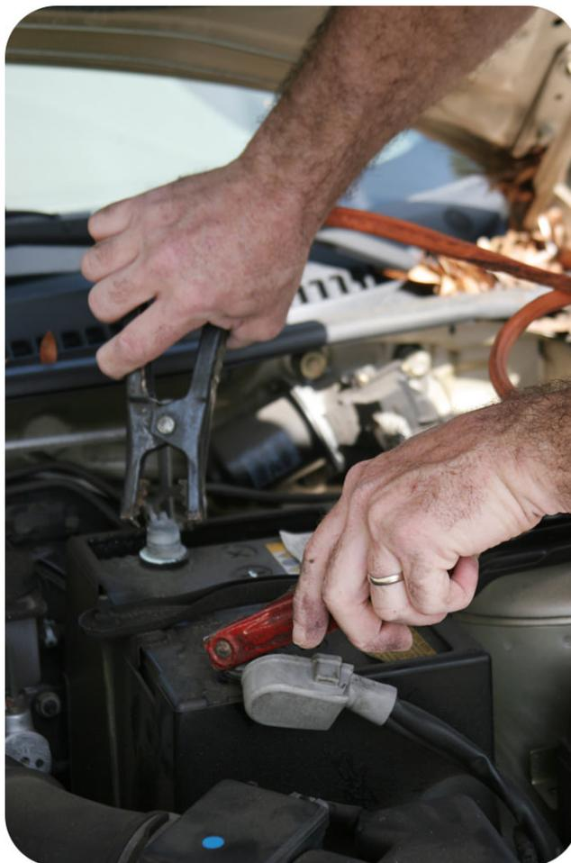
Emily's dad is giving his car battery a "jump" because the battery "died" overnight. He's attaching cables to the terminals of the car battery. Then he will connect the other ends of the cables to the terminals of a "live" battery. The cables will carry electric current to the dead battery, providing the energy needed for the car to start.
